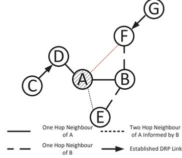
Fig. 3: Scenario with Exposed Nodes.
