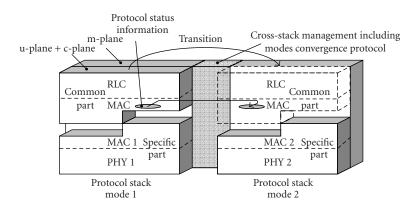
FIGURE 3: A multimode capable protocol architecture under consideration of an optimized protocol convergence. Protocol information is transferred between two modes, here exemplary depicted on the level of the MAC layer. This reflects, for instance, the case of IEEE 802.16 [3].
