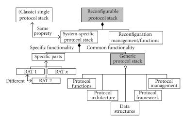
FIGURE 1: UML diagram of the generic protocol stack in the context of protocol reconfigurability.
