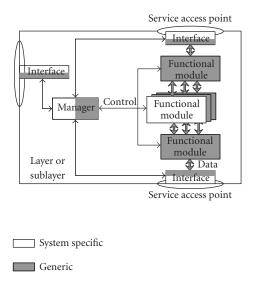
FIGURE 4: Composition of a protocol specific layer or sublayer on the basis of generic and system-specific functional modules.
