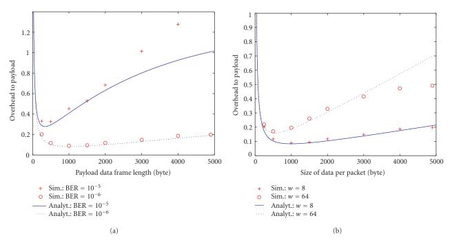
FIGURE 10: TCP layer Go-back-N ARQ validation and evaluation. The protocol overhead to payload ration in dependency on the frame length of the payload data is depicted. The lines are analytic results corresponding to (2), while the markers indicate simulative evaluation. (a) Varied BER =  $10^{-5}$  or  $10^{-6}$  and window length w = 8. (b) Varied window length w = 8 or 64 and BER =  $10^{-6}$ .
