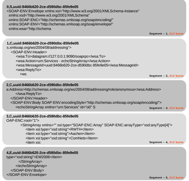
Fig. 7. Segmentation of a SOAP envelope to many datagrams with addition header information of the selective-repeat ARQ
