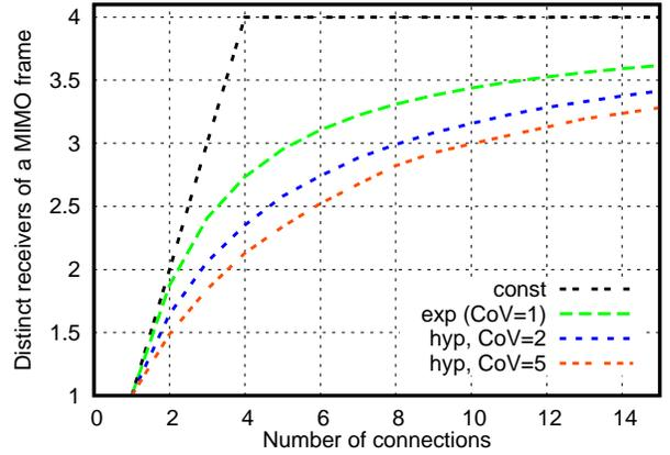
Fig. 5. Number of distinct receivers of a MIMO frame vs. number of connections for different traffic types in MU-DCF
