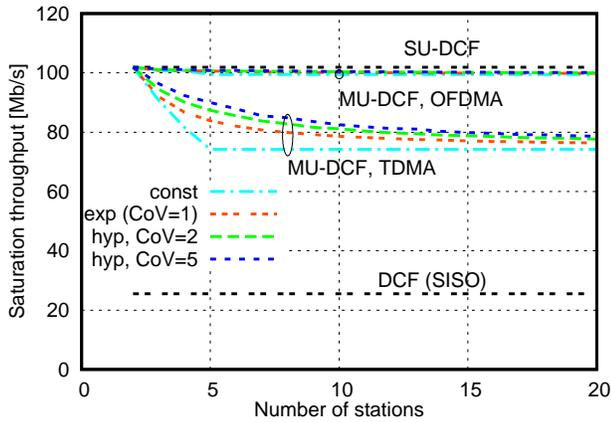
Fig. 4. Saturation throughput in Scenario I
