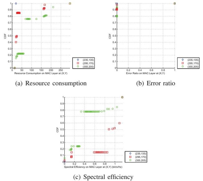
Fig. 8. CDFs of performance criteria on MAC layer at  $(X, Y)$  coordinates
