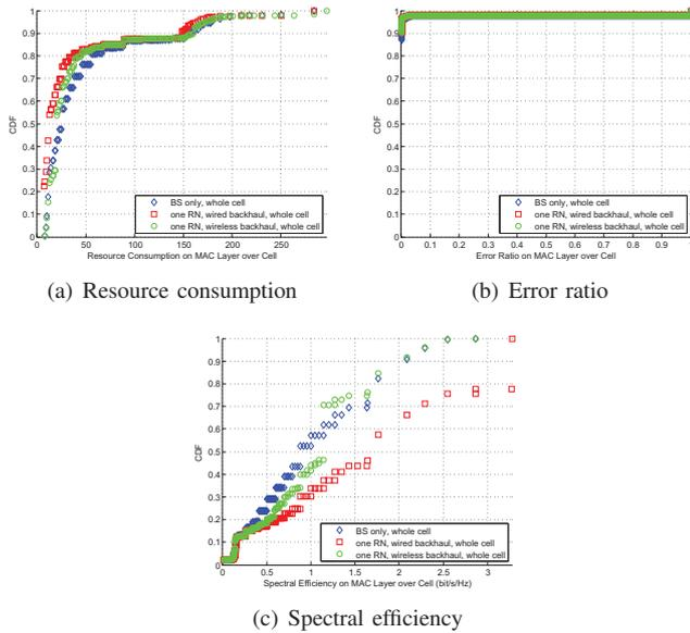
Fig. 11. CDFs of performance criteria on MAC layer in cell
