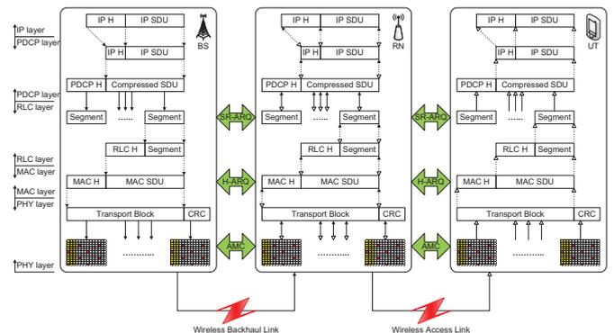
Fig. 1. Relay enhanced LTE system model
