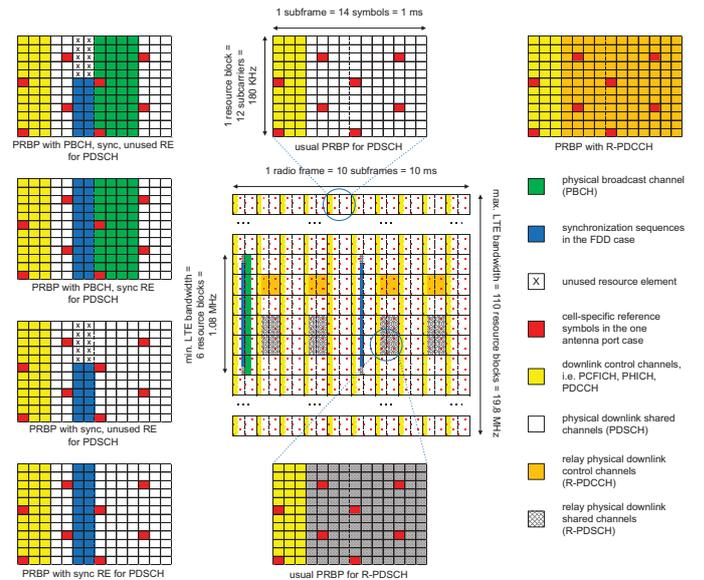
Fig. 6. LTE radio frame for relay enhanced system
