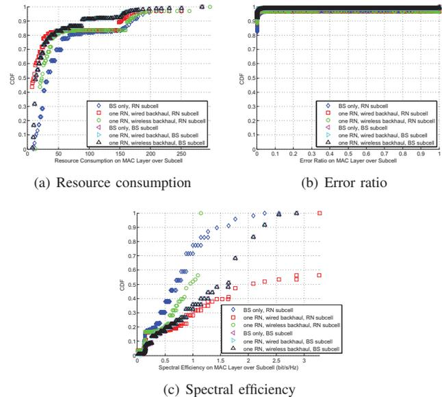
Fig. 10. CDFs of performance criteria on MAC layer in subcells
