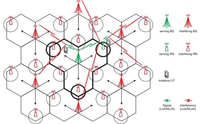
Fig. 5. Relay enhanced UMa scenario
