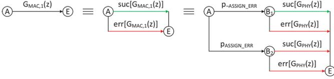
Fig. 4. SFG for MAC layer: exit condition
