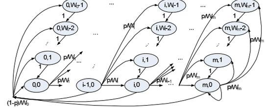
Figure 5. Bidimensional Markov chain model for DCF backoff
