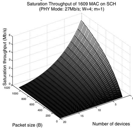
Figure 7. Saturation throughput of 1609 on SCH
