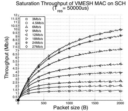
Figure 8. Saturation throughput of VMESH MAC on SCH
