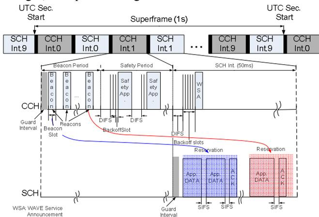
Figure 4. Channel access process of VMESH MAC
