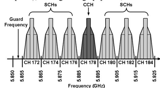
Figure 1. Frequency channel layout of 5.9GHz WAVE system
