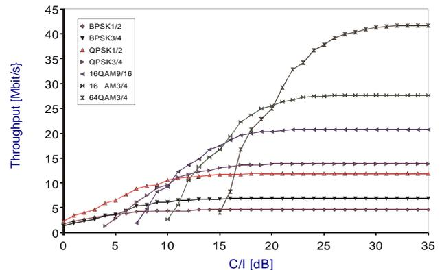
Figure 5 : Total system throughput over C/I with regard to PHY mode and ARQ
