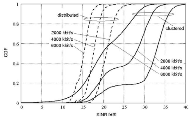
Figure 6 :  $SINR$  depending on the traffic load per downlink connection
