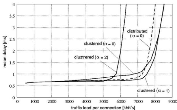
Figure 10 : Throughput-delay characteristic
