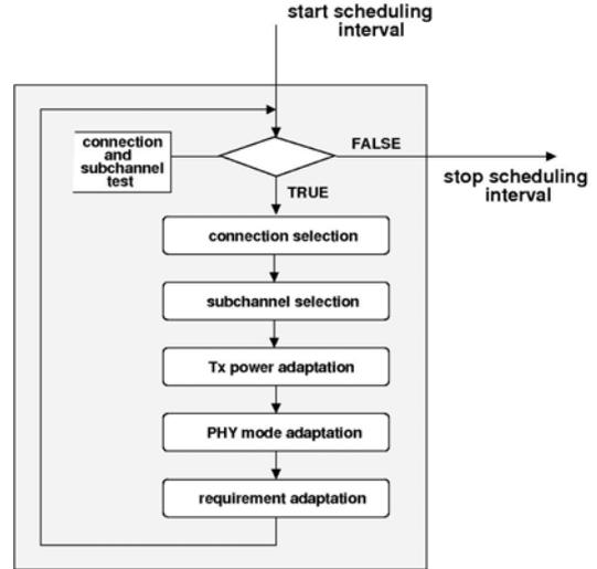
Figure 3 : Basic OFDMA scheduling algorithm
