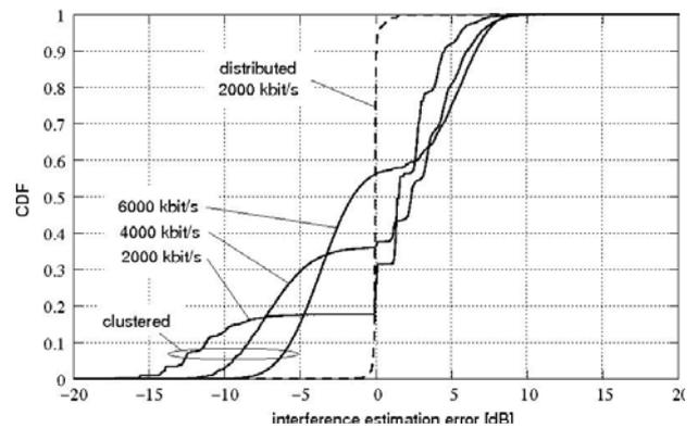
Figure 7 : Interference estimation error ( $\alpha = 0$ ) depending on the traffic load per downlink connection
