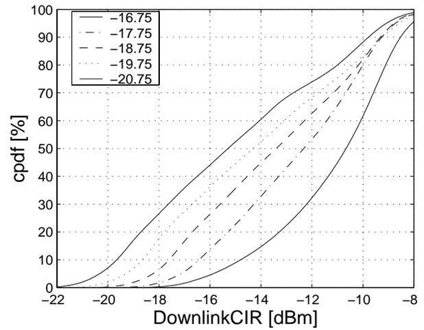
FIGURE 6 - CIR-based PC; measured CIR at the BS (UL) and UE (DL) in UTRA-FDD
