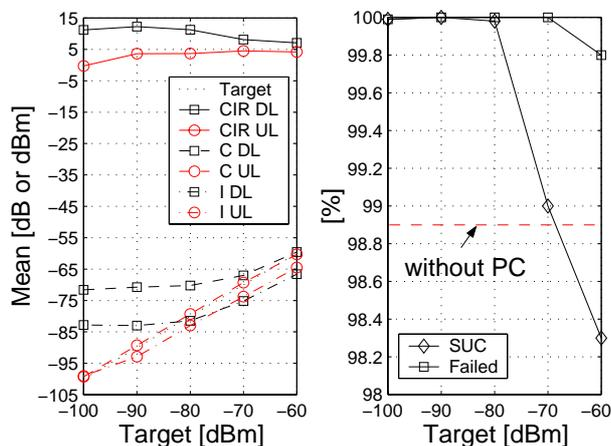
FIGURE 4 - Mean carrier (C), interference (I), CIR, and QoS at different target levels for level-based PC in UTRA-TDD
