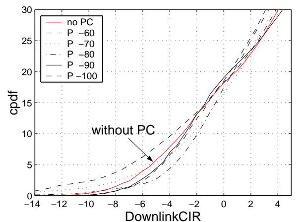
FIGURE 3 - Level-based PC; reception carrier level and CIR at the TDD UE (DL)
