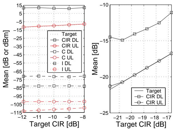
FIGURE 7 - CIR-based PC in TDD and FDD, mean values of link measurements
