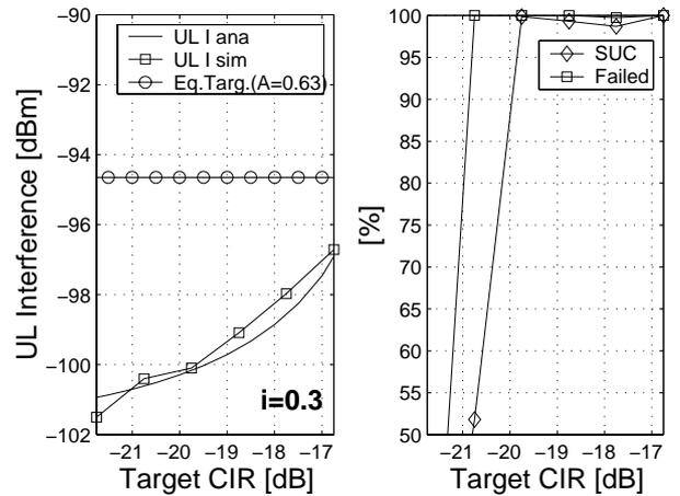
FIGURE 8 - CIR-based PC in FDD: reduction of interference and effect on QoS
