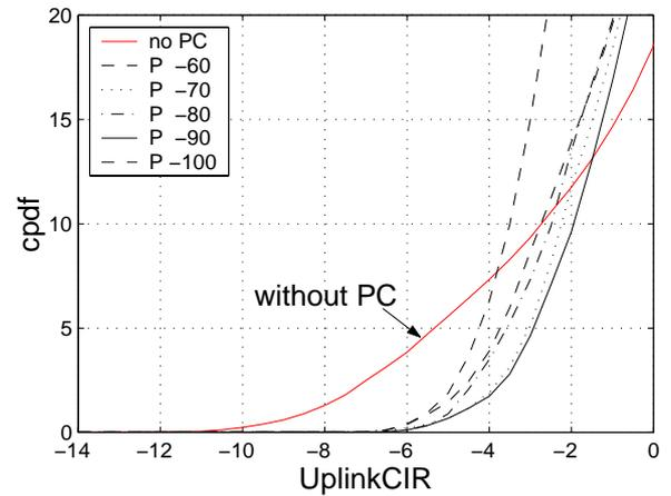
FIGURE 2 - Level-based PC; reception carrier level and CIR at the TDD BS (UL)
