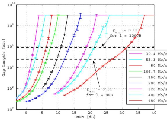
Figure 6: Average gap lengths for the average channel response of CM 1.
