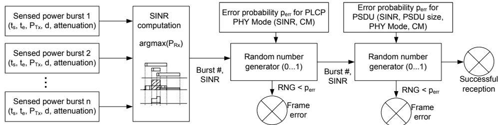
Figure 4: The stepwise error model for the UWB PHY emulation.
