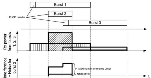
Figure 3: An exemplary SINR calculation for three concurrent transmissions.
