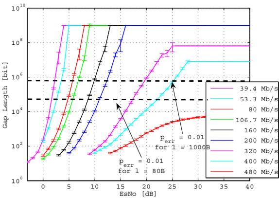
Figure 7: Average gap lengths for the average channel response of CM 3.
