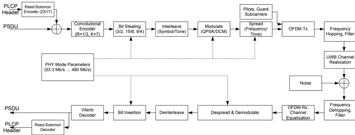
Figure 2: WiMedia PHY transmitter and receiver chain.
