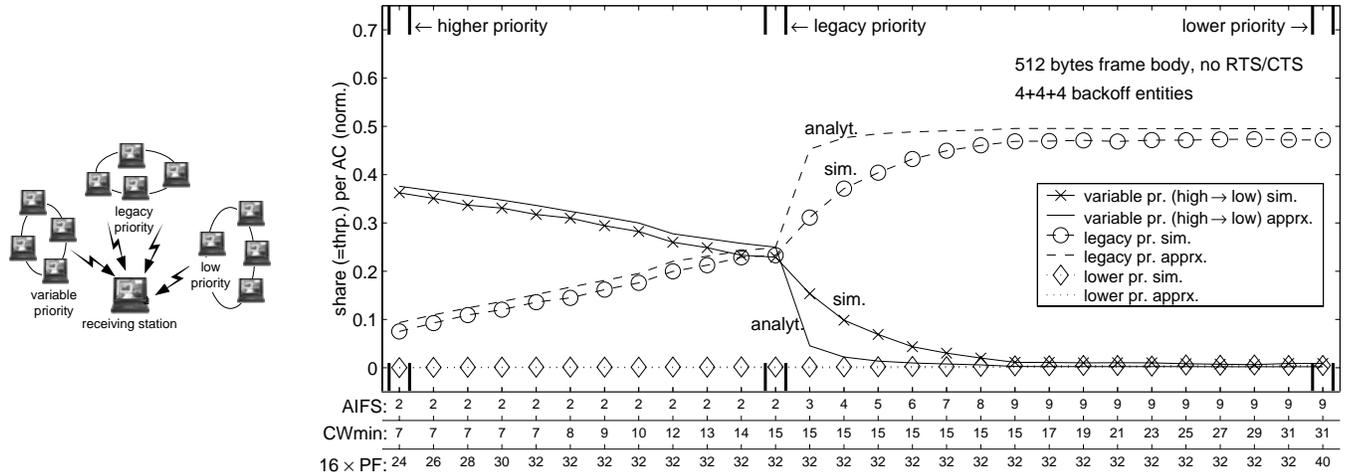
Figure 5: Scenario (left) and resulting saturation throughput per AC (right). 4 backoff entities per AC, 1 backoff entity per station. In this and all other scenarios, all stations detect each other. If two or more stations transmit at the same time, a collision occurs.
