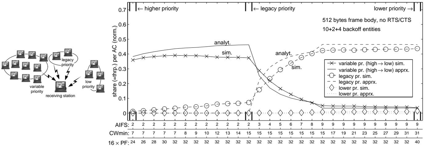
Figure 6: Scenario and resulting saturation throughput per AC. 10 backoff entities with varying EDCF parameters contend with 2 legacy and 4 lower priority backoff entities.
