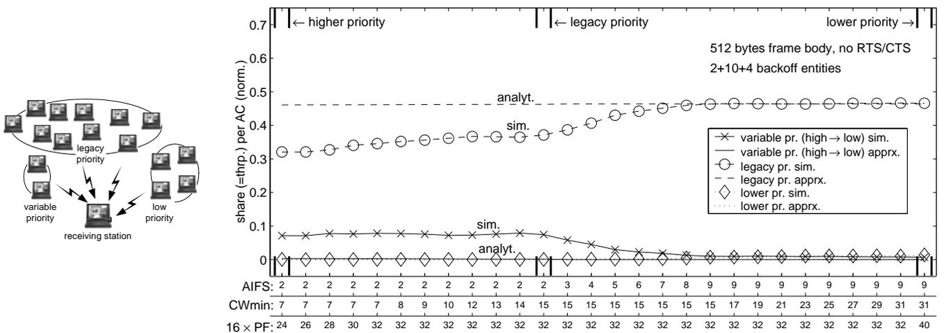
Figure 7: Scenario and resulting saturation throughput per AC. 2 backoff entities with varying EDCF parameters contend with 10 legacy and 4 lower priority backoff entities.
