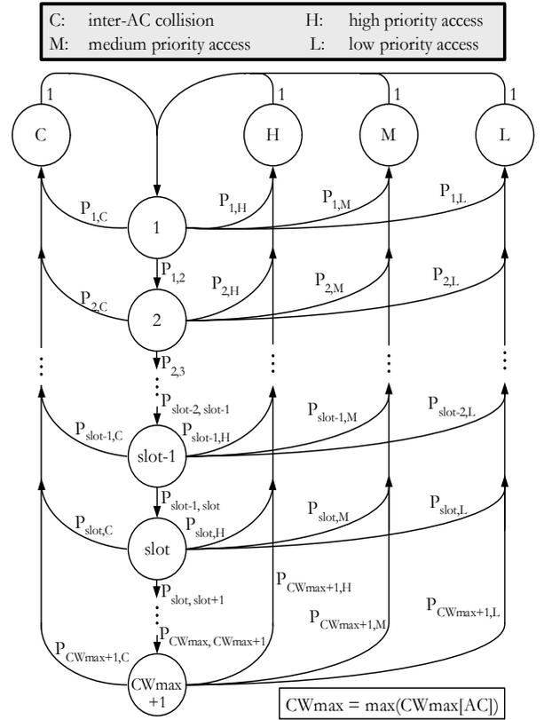
Figure 4: State transition diagram for the CSMA regeneration cycle.
