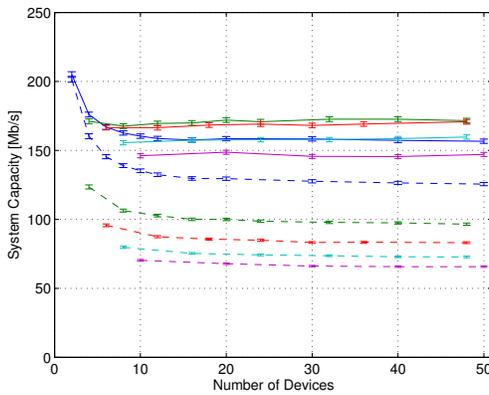
(b) Mesh points in the offices and the corridor, no forwarding functionality in the devices.
