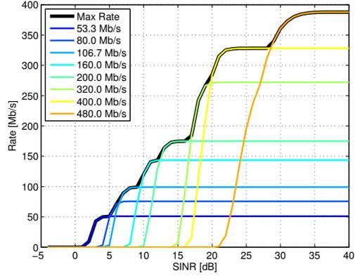
(b) Data rate versus Signal-to-Noise-plus-Interference (here for Channel Model 1 [5])
