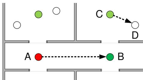
(a) Due to the wall's attenuation, A cannot hear the transmission from C to D. Hence, A starts to transmit to B, which fails due to the interference.
