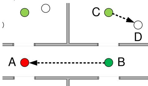
(b) Although C is transmitting to D, B could start a successful concurrent transmission to A. Nevertheless, B refrains from the medium access.
