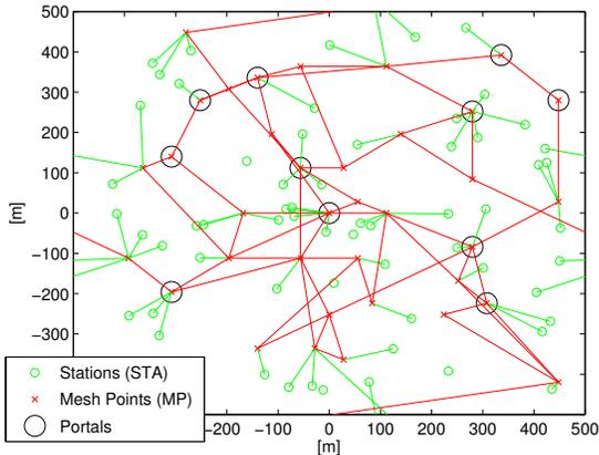
Figure 4: An exemplary instance of a mesh network with 11 portals, 24 MPs ( $r \approx 2.2$ ) and 50 STAs.
