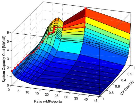
Figure 8: System capacity cost; the cost of a portal is normalized to 1\$. The maximum system capacity cost for each MP value is given by the red line.
