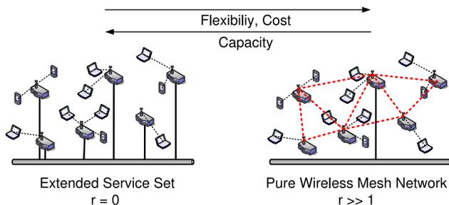
Figure 1: The coverage of IEEE 802.11 can be extended using a wired (ESS) or a wireless (mesh) backbone. The possible solution space in between is characterized by the ratio  $r$  of mesh points per portal.
