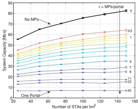
Figure 7: System capacity for different ratios  $r$  and number of served STAs.
