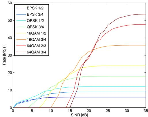
Figure 3: For a chosen Modulation- and Coding Scheme (MCS), the Signal to Interference plus Noise Ratio (SINR) determines the final transmission rate.
