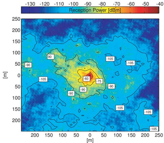
Figure 2: Reception power (in dBm) from a sender positioned at the center of the area.
