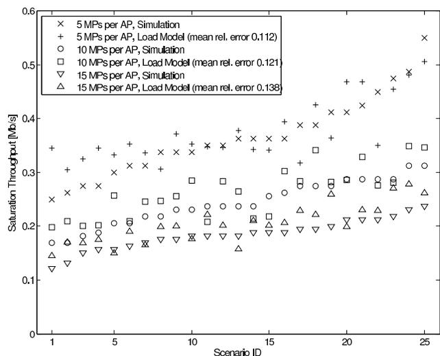
Fig. 2: Saturation throughput of 75 different scenarios, computed using the IEEE 802.11 model and event-based simulation as reference.
