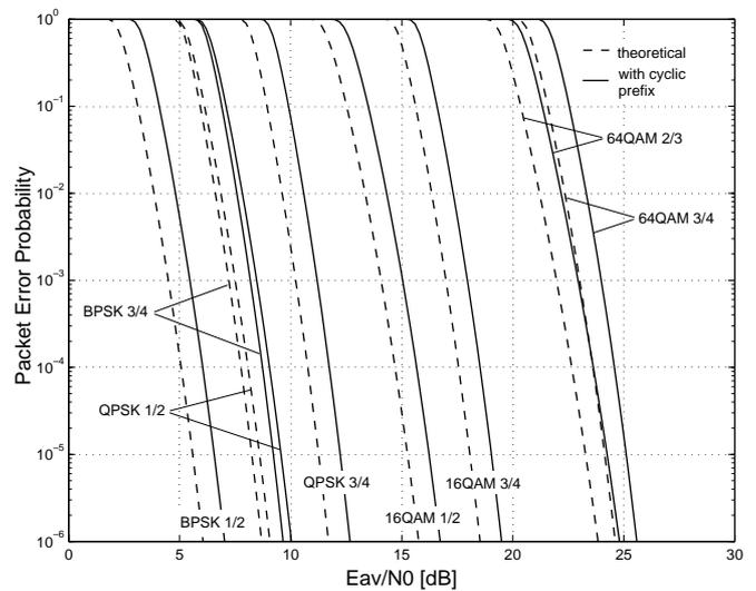
Figure 4. Theoretical PER for a 1514 byte long packet. The solid lines refer to a multicarrier system with  $a_{cp} = 80\%$ .
