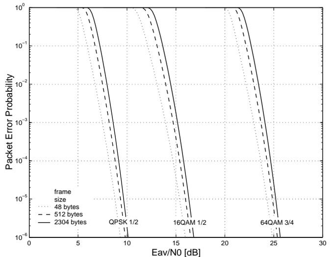
Figure 5. PER vs.  $E_{av}/N_0$  for different packet sizes
