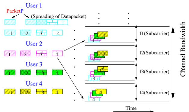
Figure 1. MC-CDMA principle with SF= 4
