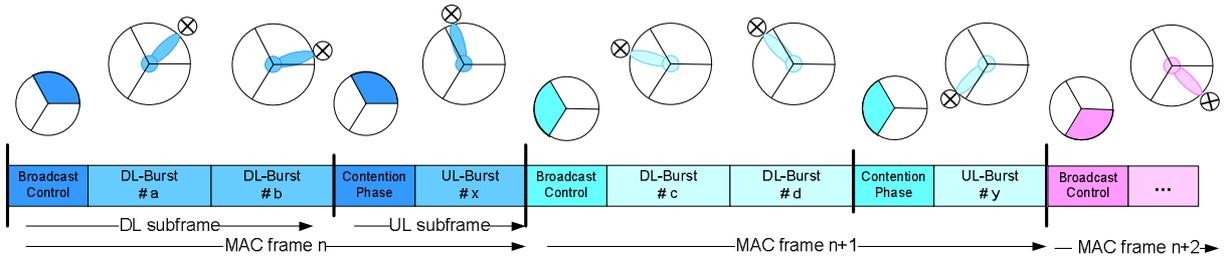
Figure 4. MAC frame and corresponding antenna pattern of space-time sectorization scheme
