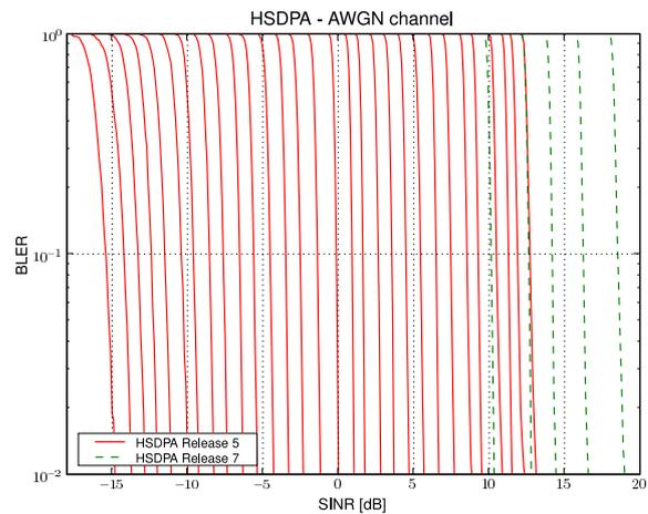
Figure 1: HSDPA BLER mapping for an AWGN channel
