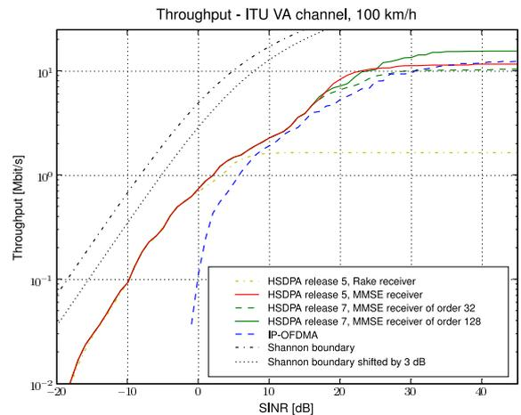
Figure 5: Throughput for ITU VA channel, 100 km/h
