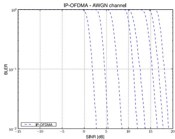
Figure 2: IP-OFDMA BLER mapping for an AWGN channel
