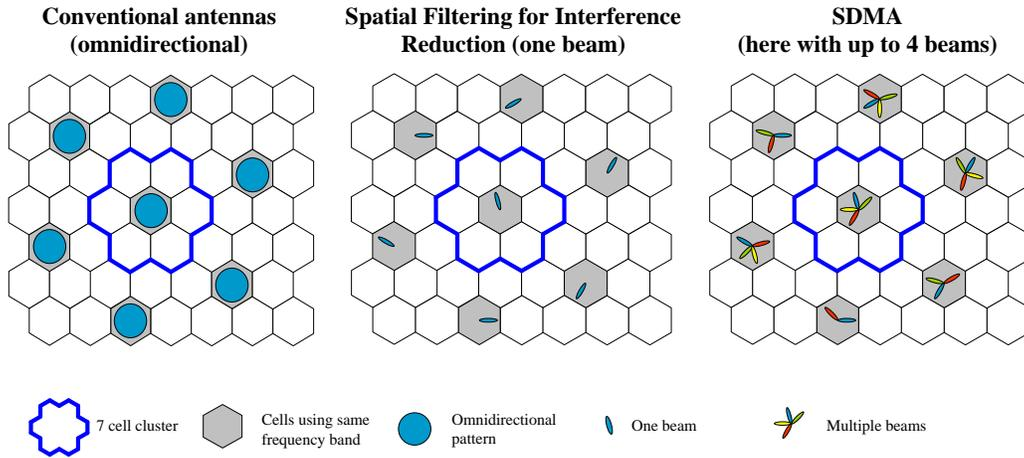
Fig. 2. Comparison of a 7 cell cluster with omnidirectional and beamforming antenna in SFIR and SDMA mode. Adapted from [9].
