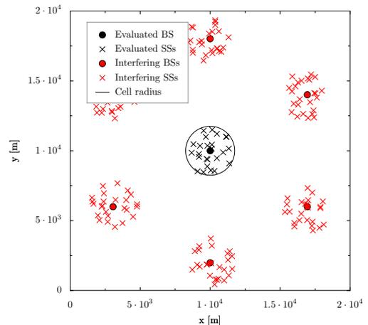
Fig. 3. Positions of BSs and SSs in central (black) and co-channel (red) cells of evaluated clustered cellular deployment
