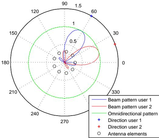
Fig. 1. Radiation pattern for 9-element circular antenna arrays (algorithm, see: [8])
