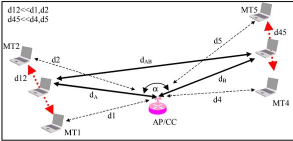
**Figure 3: Self-interference for SDiL appliance**
