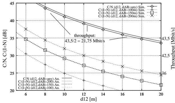
**Figure 5: Signal quality for DiL (C/N) and SDiL (C/(I+N)) as a function of the terminal distance  $d_{12}$**
