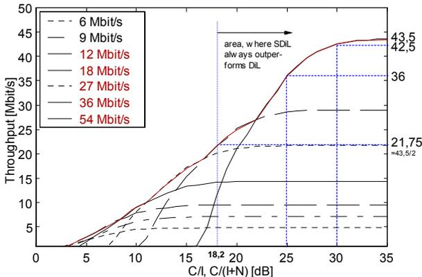
**Figure 4: H/2 max. system throughput for resp. Phy-modi**
