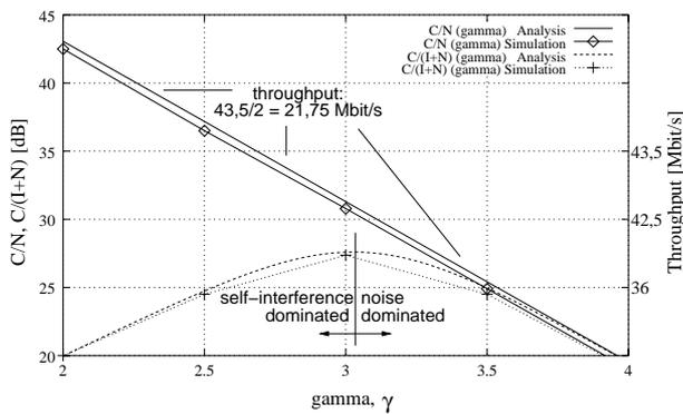
**Figure 6: Impact of the propagation coefficient  $\gamma$  on the signal quality for DiL (C/N) and SDiL (C/(I+N))**
