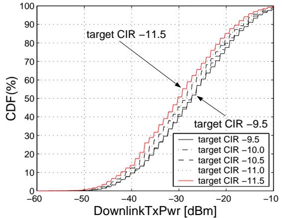
**FIGURE 9 – Downlink Tx power distribution**
