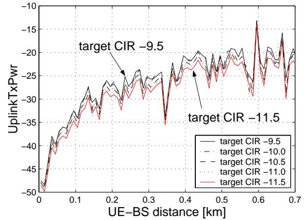
FIGURE 14 – Uplink Tx power over distance.
