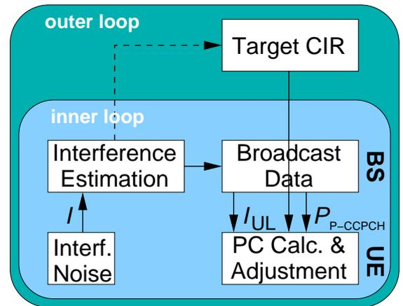
FIGURE 1 – Open loop PC in uplink.
