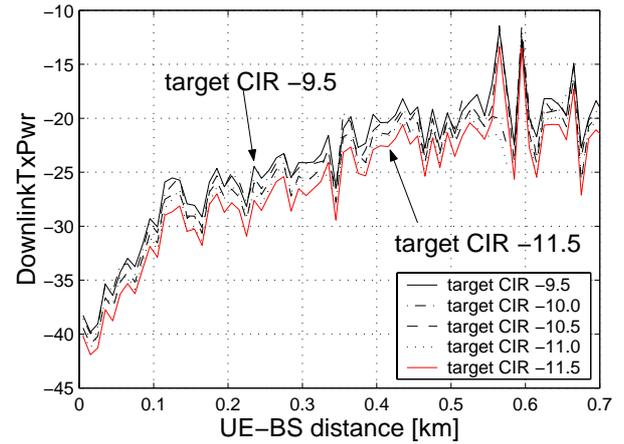
FIGURE 13 – Downlink Tx power over distance.
