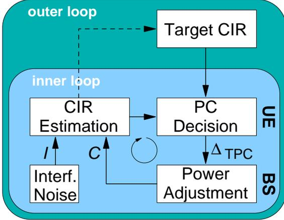
FIGURE 2 – Closed loop PC in downlink.
