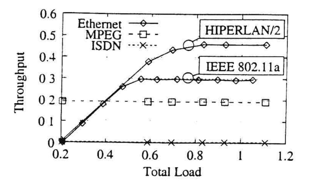
Fig. 18. Relative throughput of the traffic flows.
