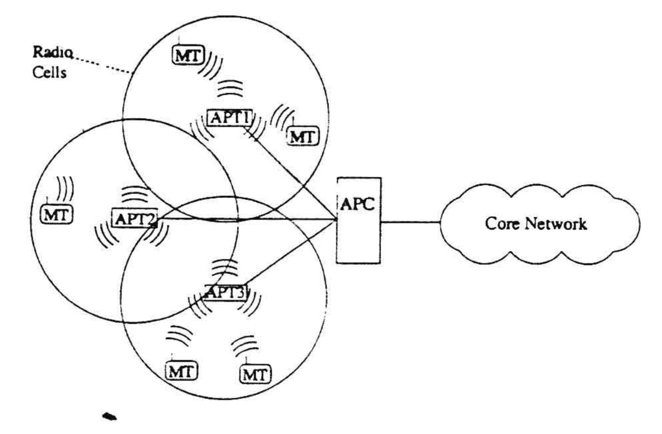
Fig. 2. Structure of a cellular H/2 system
