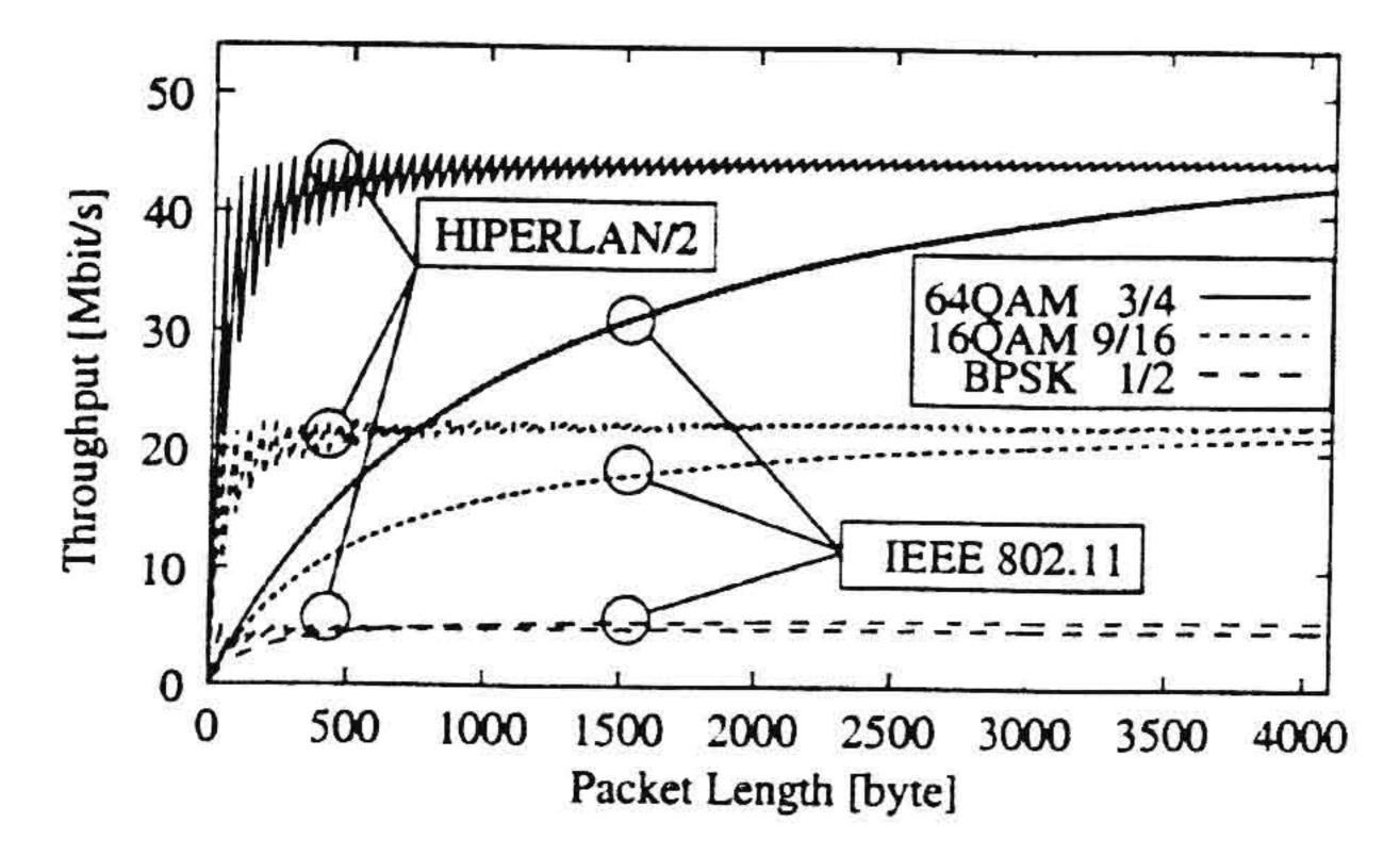
Fig. 16. Throughput over packet length.
