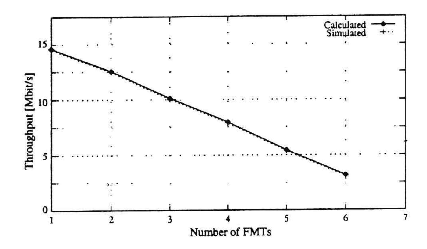
Fig. 36. Maximum AP-to-RMT throughput versus number of FMTs.
