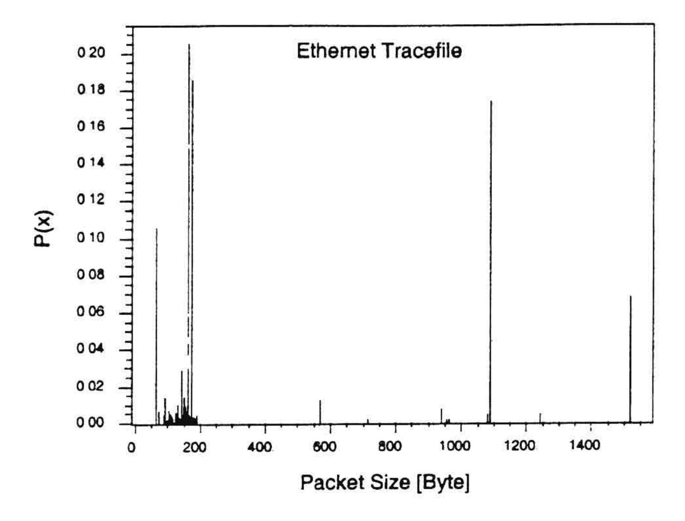
Fig. 12. Ethernet packet length distribution.
