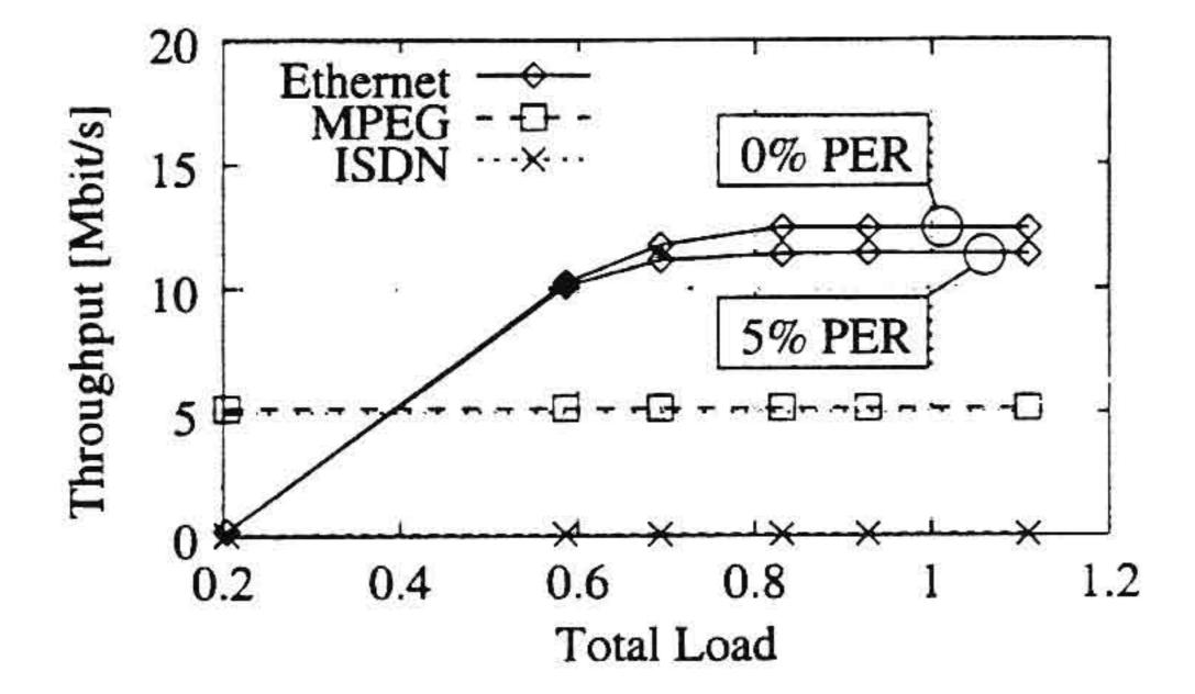
Fig. 20. Throughput of the traffic flows, with PER = 5%
