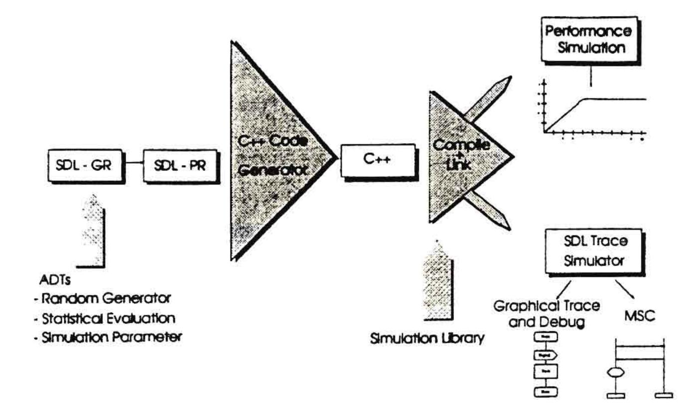
Fig. 11. Creation of a simulation.
