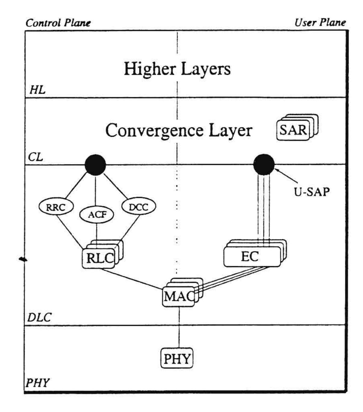
Fig. 4. Service model of H/2.
