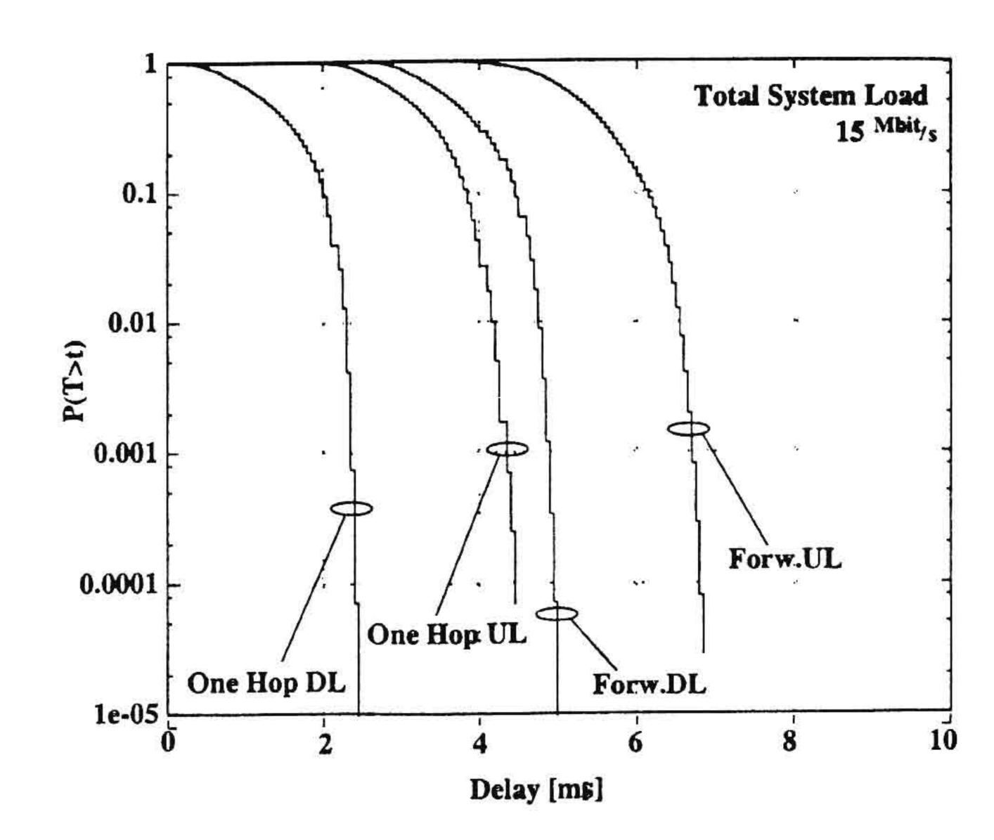
Fig. 37. CDF of delay under forwarding.
