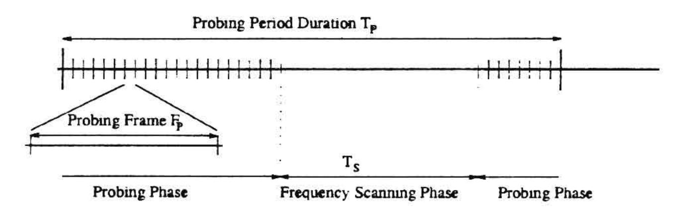
Fig. 25. CC probing period of a CC-capable terminal
