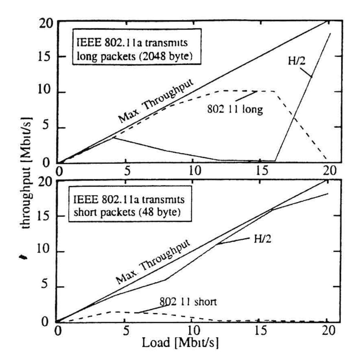
Fig. 22. Throughput of H/2 and IEEE 802 11a versus load
