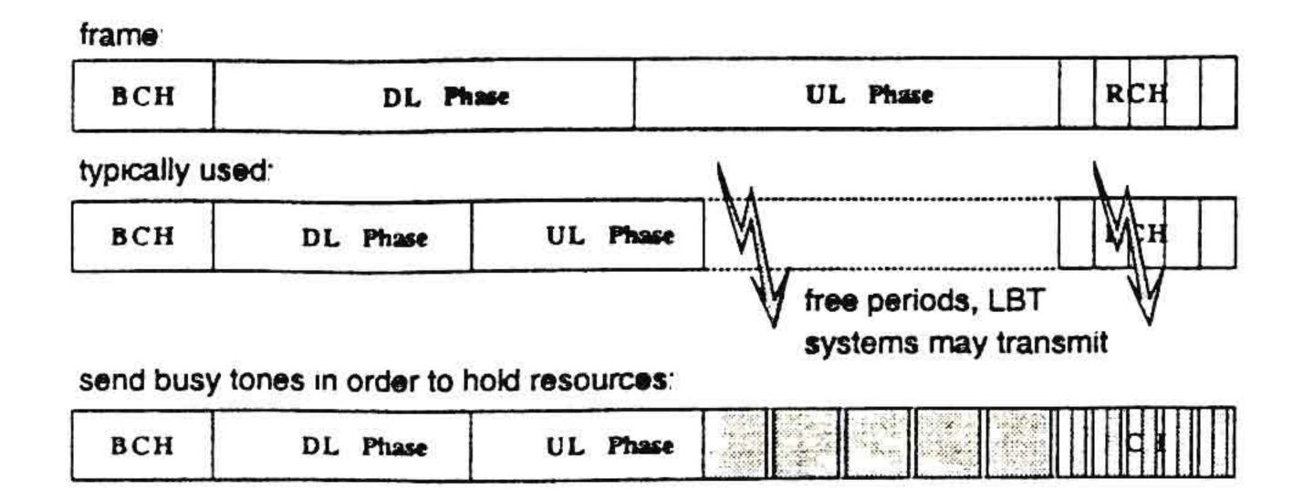
Fig. 23. Interference protection by filling up the H/2 MAC frame.
