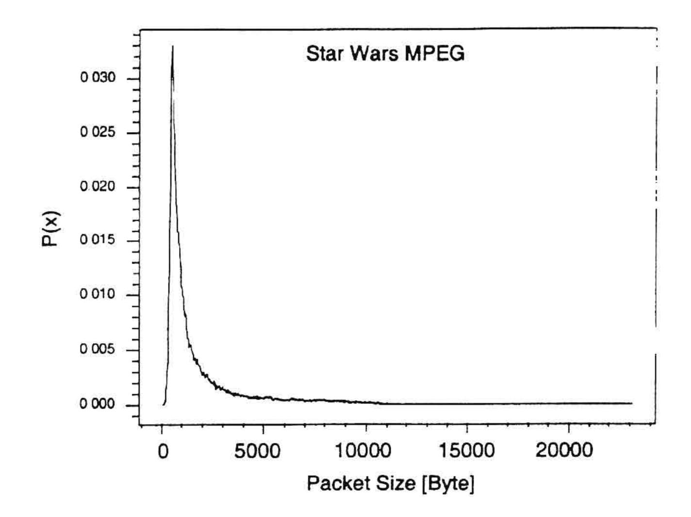
Fig. 13. MPEG packet length distribution
