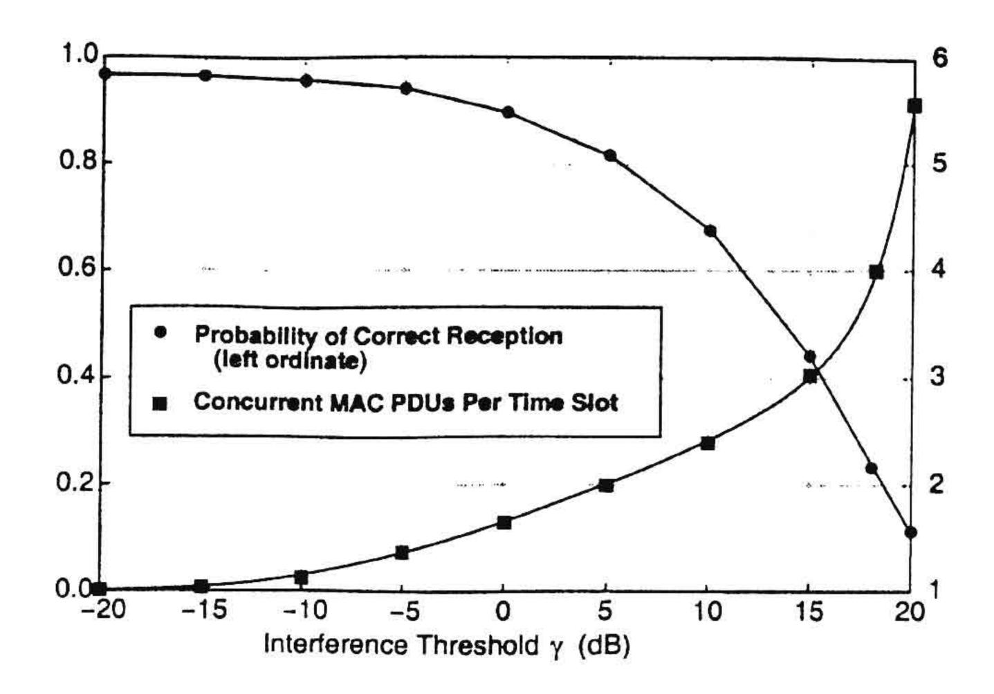
Fig. 31. Successful reception and spatial exploitation for k = 6 MTs.
