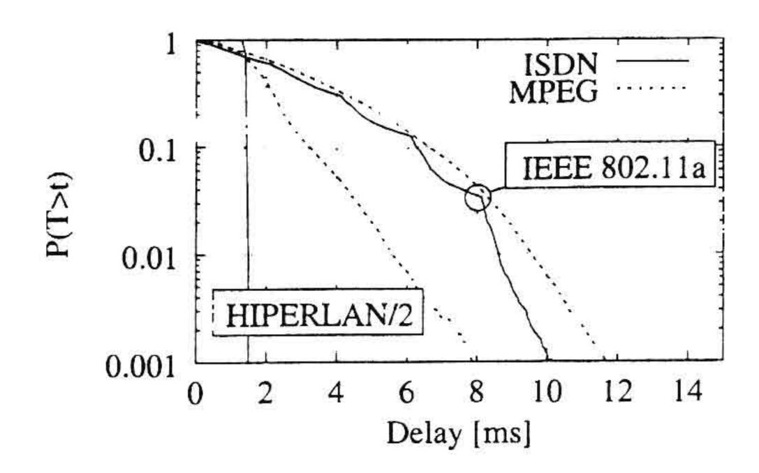
Fig. 19. CDF of the user packet delay
