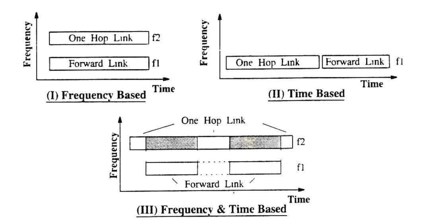
Fig. 33. Forwarding concepts in time and frequency domains
