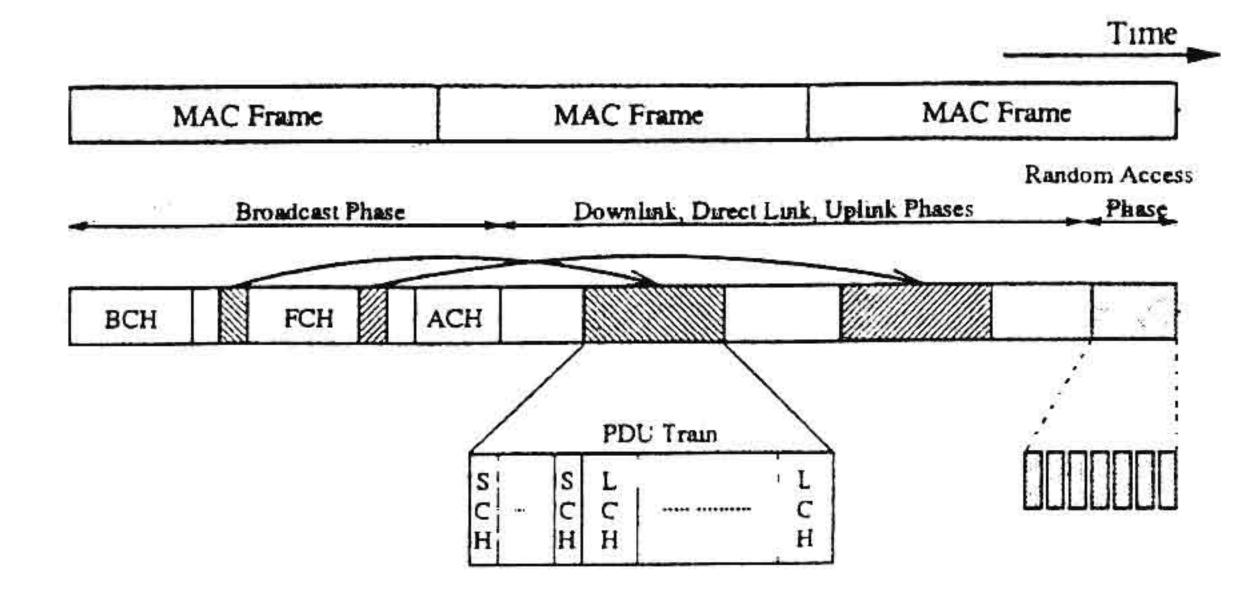
Fig. 6. Transmission phases in a MAC frame
