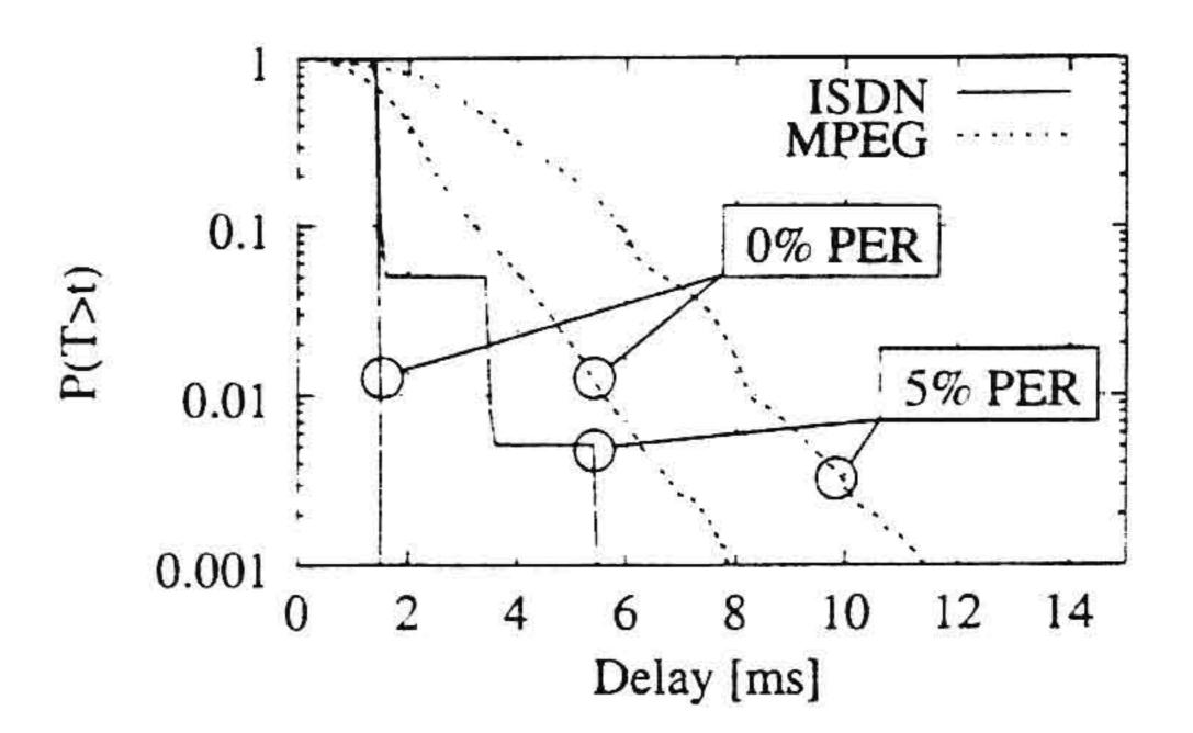
Fig. 21. CDF of the packet delay, with PER = 5%.
