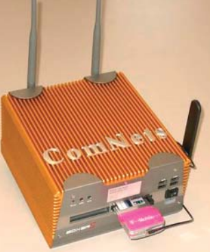
Figure 1: Product Prototype of the Vehicular Communication Gateway
