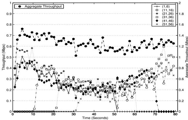
Figure 19: The throughput trace of each TCP connection and their aggregate value over the grid topology. The TCP connection changing pattern is specified in Fig.21, VTT=120, Cwnd=20, MaxTCH=2. Throughputs are measured every 1.2 s.
