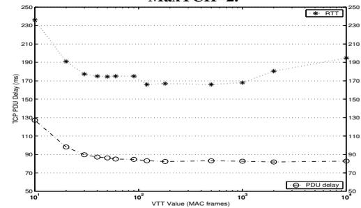
Figure 14: Impact of VTT on TCP PDU delay, Cwnd=20, MaxTCH=2.
