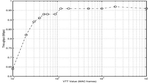
Figure 13: Impact of VTT on TCP throughput, Cwnd=20, MaxTCH=2.
