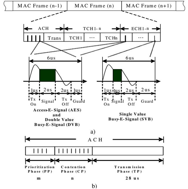
Figure 2: a) MAC frame and waveforms of energy signals; b) ACH structure.
