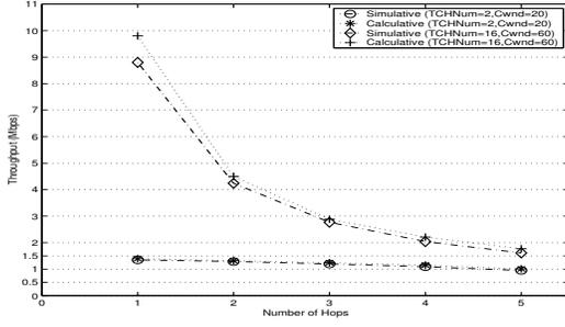
Figure 7: TCP throughput over the string network, VTT=120.
