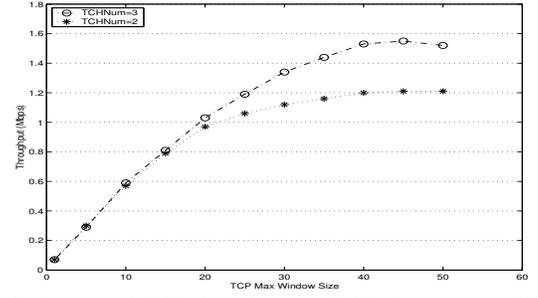
Figure 9: Impact of TCP Cwnd on the TCP throughput, VTT=120.
