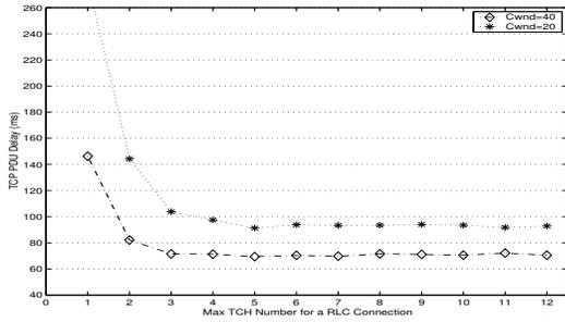
Figure 12: Impact of the maximum TCH number for an ARQ connection on TCP PDU delay, VTT=120.
