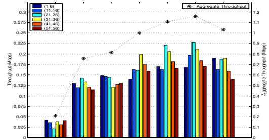
Figure 17: Impact of VTT on throughput over the grid topology, Cwnd=20, MaxTCH=2.
