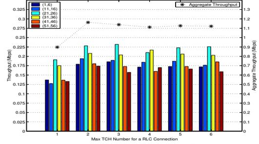
Figure 16: Impact of the maximum TCH number for an ARQ connection on throughput over the grid topology, VTT=120, Cwnd=20.
