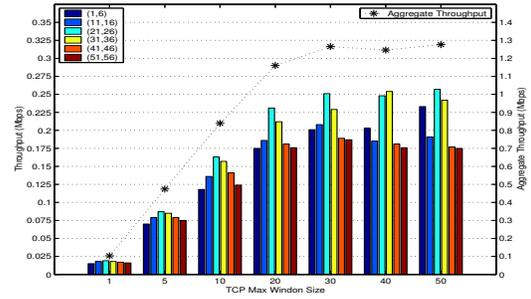
Figure 15: Impact of TCP congestion window size on throughput over the grid topology, VTT=120, MaxTCH=2.
