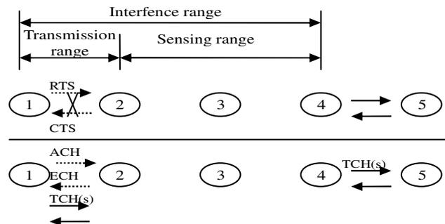
**Figure 4: An example of transmission in multi-hop networks. Node 1 wants to setup a connection with node 2 while a transmission is ongoing between nodes 4 and 5.**
