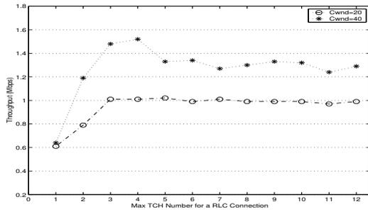
Figure 11: Impact of the maximum TCH number for an ARQ connection on TCP throughput, VTT=120.
