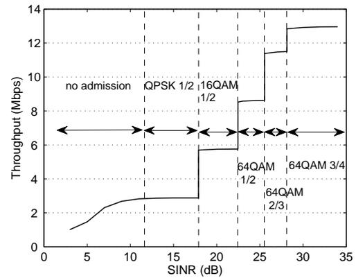
**Figure 3. Max. achievable throughput at PER threshold of 1 %**
