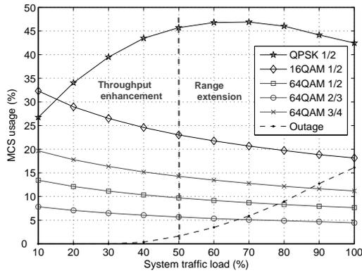
**Figure 12. MCS usage in a non-relay cell vs. system traffic load**
