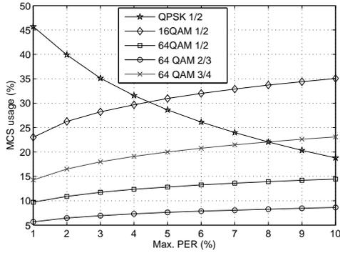
**Figure 8. MCS usage vs. PER threshold in a non-relay cell. Cell radius=500m**
