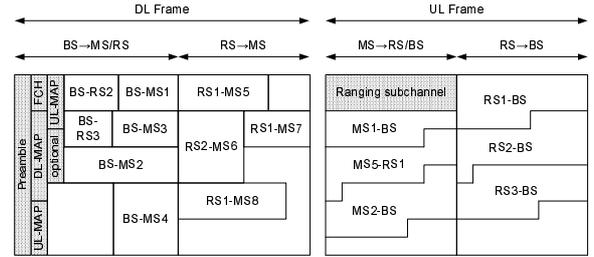
**Figure 2. OFDMA frame structure with two-hop transmission capability [12]**
