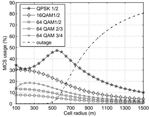
Figure 4. MCS usage in a non-relay cell
