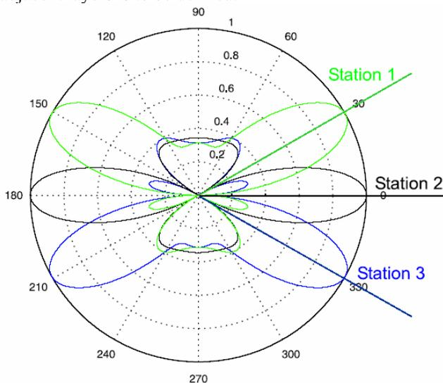
Figure 8: Three beam patterns of a 4-element ULA
