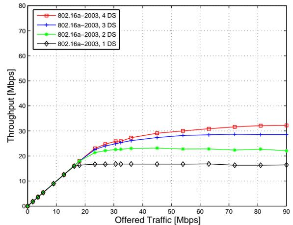
Figure 12: System throughput of IEEE 802.16a-2003
