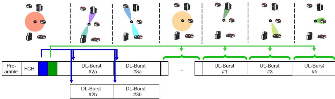
Figure 11: SDMA support of IEEE 802.16a-2003
