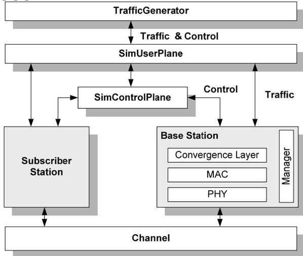
Figure 5: Structure of SDL-based simulator
