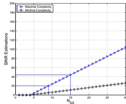
Figure 22: Computational complexity of the simplified SDMA scheduler
