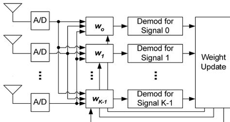
Figure 2: Beamformer for multiple signals
