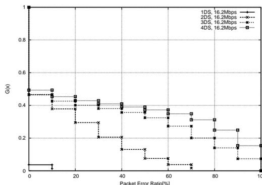
Figure 18: CDF of packet error ratio
