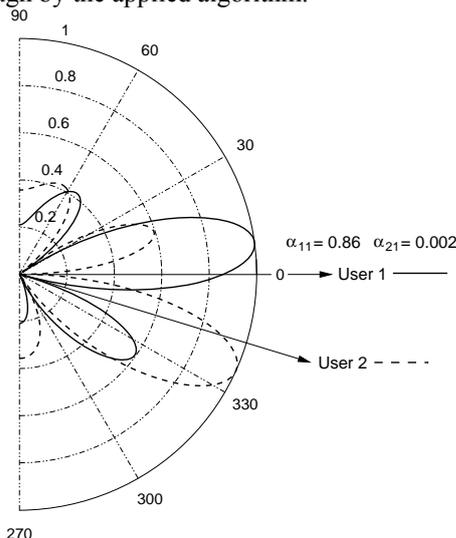
Figure 3: Two optimized beam patterns and corresponding amplitude factors ( $\alpha$ )
