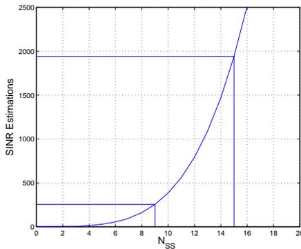
Figure 20: Computational complexity of the Max Throughput SDMA scheduler
